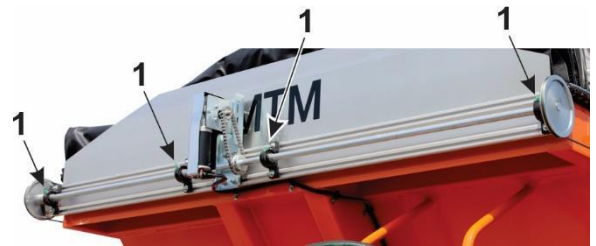
(1078) Figure 4-10 g – Slide Tarp Drive System Lubrication
