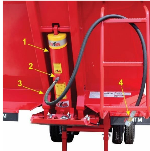
Figure 4-4 – Hydraulic Cylinder and Hydraulic Hose Inspection
