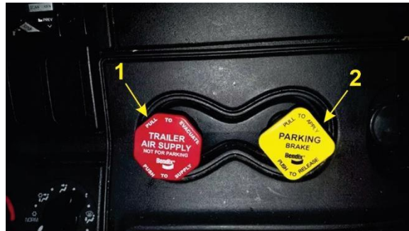
Figure 4-8 – Tractor Air Supply Controls
