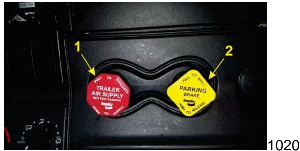
Figure 4-16 – Tractor Air Supply Controls
