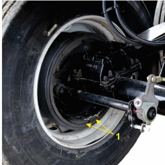
(1033) Figure 4-9 – Brake Lining Inspection
